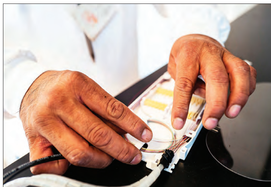
Saddleback Communications Commercial Tech II Ron Thomas demonstrates how to splice fiber.
