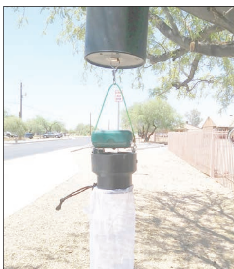
An EVS mosquito trap set out for the night, usually hanging from a tree. This trap emits carbon dioxide from dry ice, which attracts the mosquitoes.
