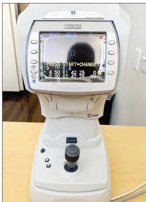
This three-in-one machine is non-contact auto retorefractor, autokeratometer, and non-contact tonometer, this new device helps optometrist get non-invasive and quicker results to patients.
