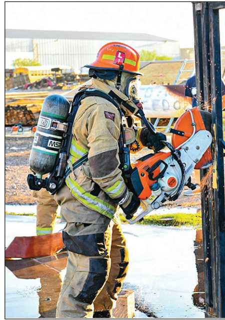
Daniel Garcia uses a STIHL TS 700 Quicksaw to break open a door in his timed exercise.
