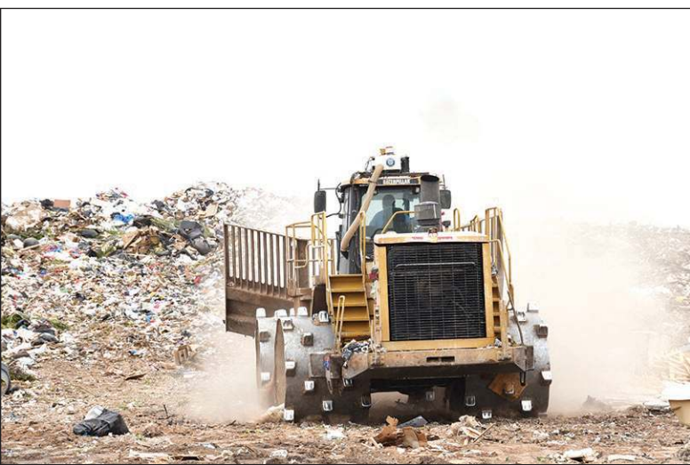
A compactor levels solid-waste at the Salt River Landfill.
