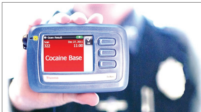
A police officer holding a TruNarc device that is detecting an illegal substance. Photo courtesy of SRPD
