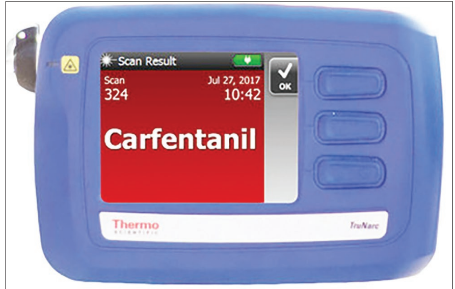
A photo of a TruNarc device detecting the substance carfentanyl. Photo courtesy of SRPD
