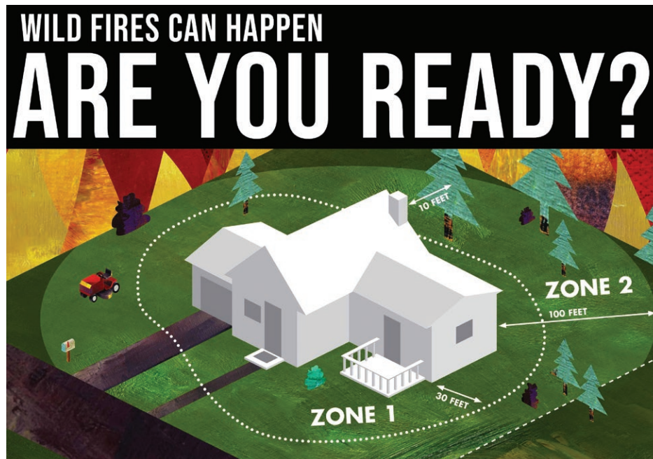
In Zone 1 keep up to 30 feet of your home clear of any vegetation or other items that could catch fire, Zone 2 extends from 30 feet to 100 feet out from your home to your property line; keep your lawn mowed, remove fallen leaves, twigs, bark and small branches to help prevent the spread of a brush fire.
