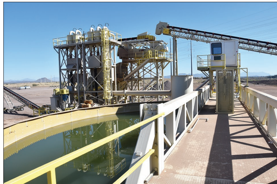
The wash plant, where different materials such as rock and sand granules of different sizes are sifted and broken down.
