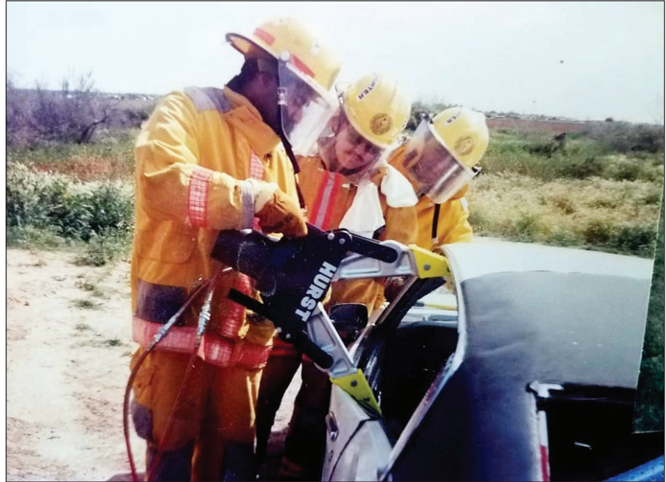
Odie working on a vehicle extrication and opening a door with a Hurst hydraulic spreader tool behind Station 291 in 1993. The middle firefighter is Rick Dodge and the firefighter to the right is Forrest Anton. Photo courtesy of Odie Toney
